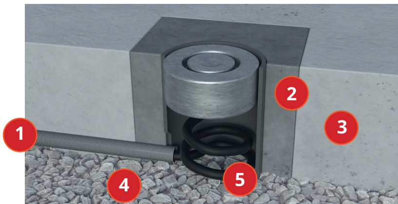
An example of installing a temperature and moisture sensor in the pavement
